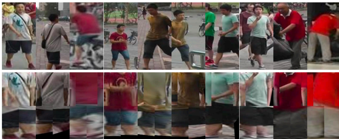
Figure 1. Examples of misalignment correction by PoseBox. Row 1: original bounding boxes with detection errors/occlusions. Every consecutive two boxes correspond to a same person. Row 2: corresponding PoseBoxes. We observe that misalignment can be corrected to some extent.
